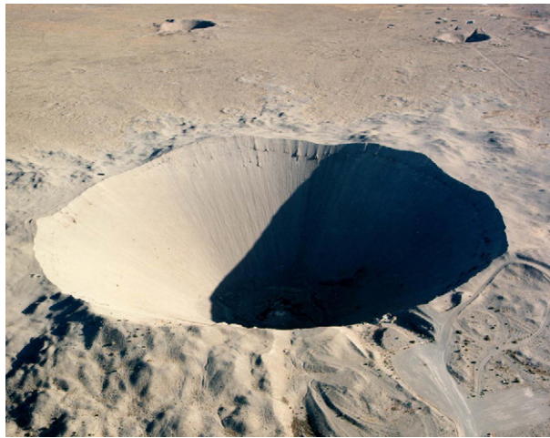
Figure 4 Project Plowshare experimental blasts were conducted from 1961 to 1973 for peace-time tests of the feasibility of effecting geomorphic changes for construction. The Sedan crater was produced by a test nuclear detonation of 104 kilotons at the Nevada Test Site in 1962. The blast is 98 m deep and 390 m in diameter. Source: US Department of Energy, 2000. United States Nuclear Tests, July 1945 through September 1992. Nevada Operations Office, DOE/NV-209-REV15.
